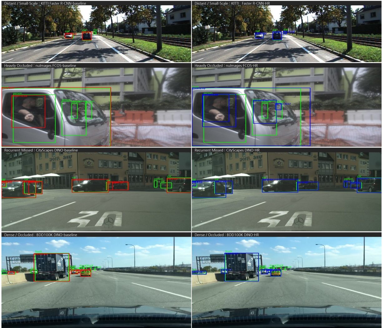
Figure 6: Qualitative detection comparison between the No-HR baseline (left) and validation-selected Hard Replay (right). Green boxes denote ground truth; red boxes are baseline predictions and blue boxes Hard Replay predictions, with confidence labels. Rows are organized by failure mode, named in each row header. Selection criterion and split are given in Section 4.5 .
