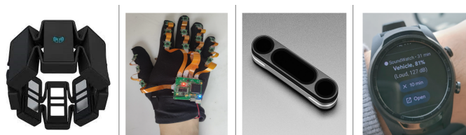
FIGURE 4. Types of sensor devices applied in the collection of sign language data (a) Myo armband [82] (b) Data gloves [81] (c) Ultraleap Motion [83] (d) SoundWatch [84].
