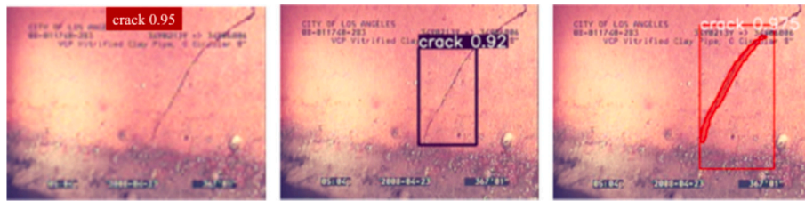
Fig. 3. Example of sewer pipeline crack inspection using image classification (left), object detection (middle) and image segmentation (right) [28].
