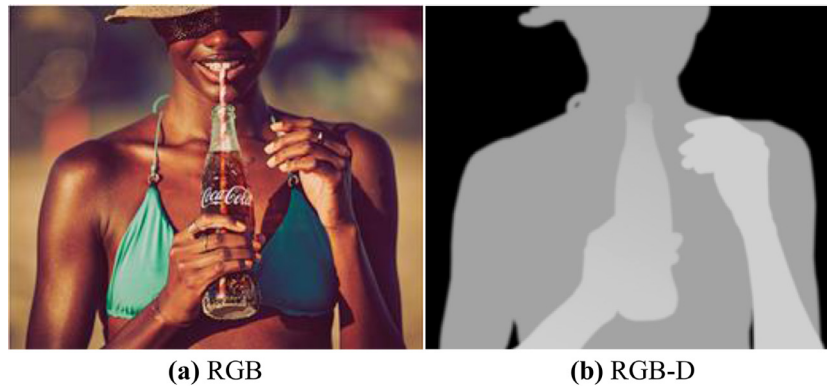
Fig. 4. Comparison of the two types of data, (a) RGB image and (b) RGB-D that contains the corresponding depth data for the RGB. In an RGB-D image, each pixel indicates a distance between the screen space and an object in the RGB image. Bright pixels, which are close to the camera, are having the highest value, and dark pixels, which are far from the camera, are having the lowest values.
