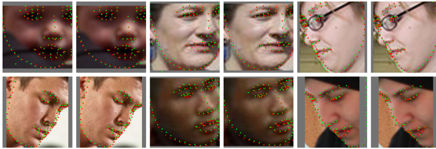
FIGURE 3. Visualization of Landmark detection result. Image pairs are displayed side by side for comparison. Left images: result from heatmap model (HRNet18). Right images result from GCN landmark model. Green dot: predicted landmark location. Red dot: groundtruth landmark location.
